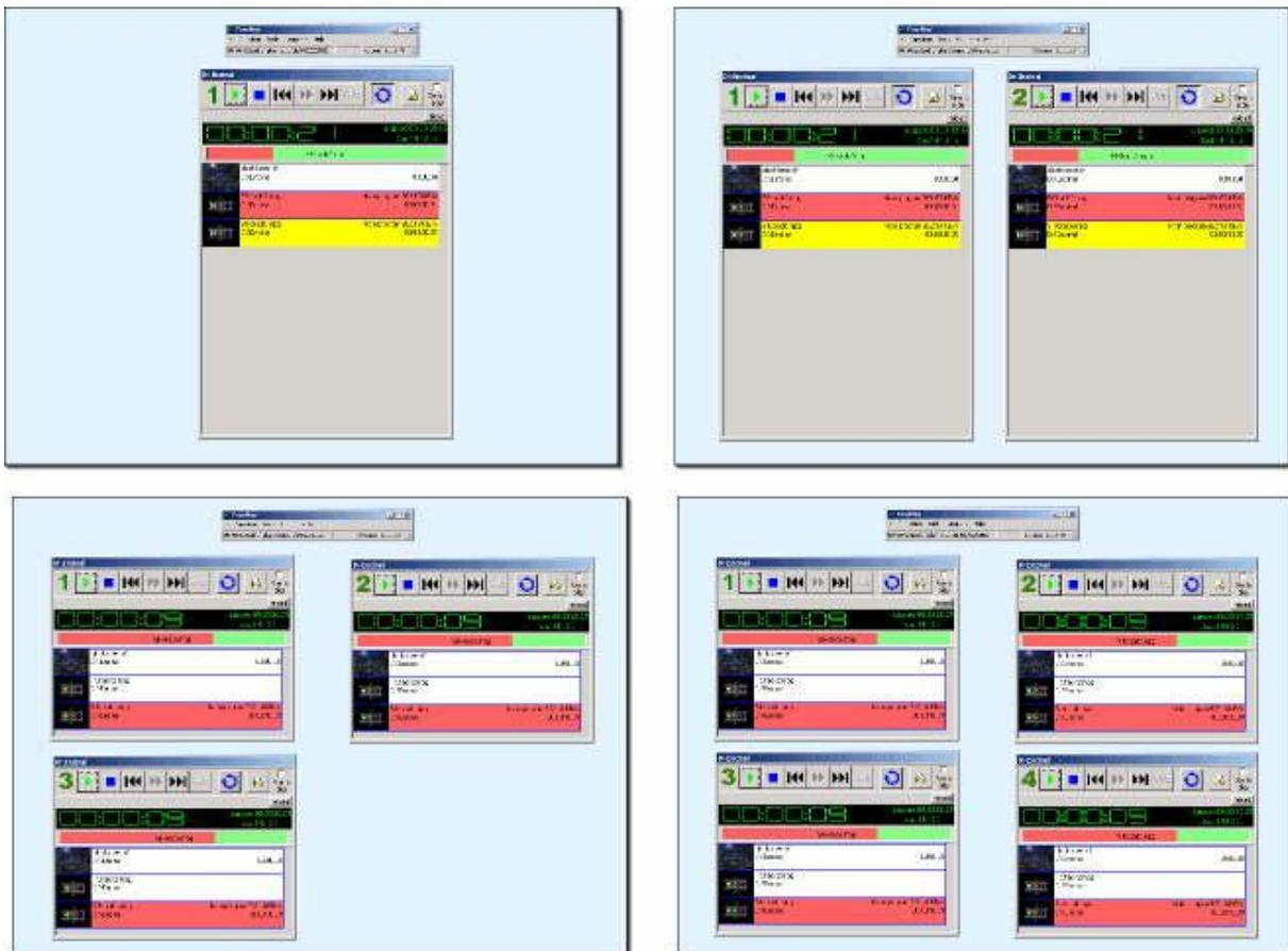
NOTE: To position the windows as shown, click **Configuration** in the EasyPlay menu bar and select **Rearrange window**. You can modify the placement and cropping at any time. If you want to keep the modifications, click **Save window parameter**. The next time you open the program, the windows will appear in the saved positions.
